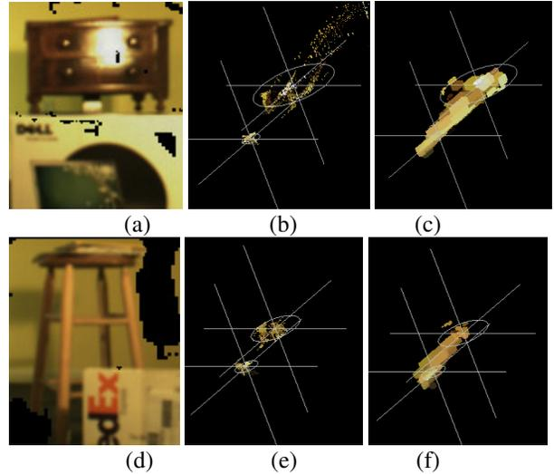
**Figure 2:** Occluded Landmark left image of stereo pair (a, d); perspective view of image pixels mapped to absolute depth (b, e); perspective view of terrain spatiogram with XZ cluster center and 1SD circle (c, f).
