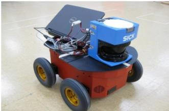
**Figure 6.** Pioneer 3-AT Robot used in both Missions
