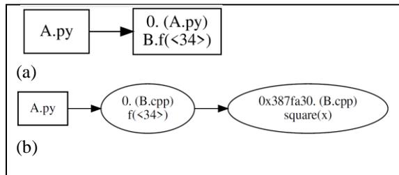
**Figure 4:** Multilingual call-graph extracted by MLSA from the example in Fig. 2: (a) just A.py and (b) for A.py and B.cpp/.h *Node shape: Rect: Python; Ell: C/C++.*
