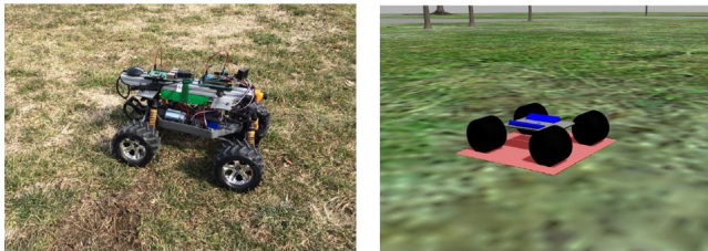
Fig. 1: Modified Traaxis platform used in field trials (left); simulation model (right).
