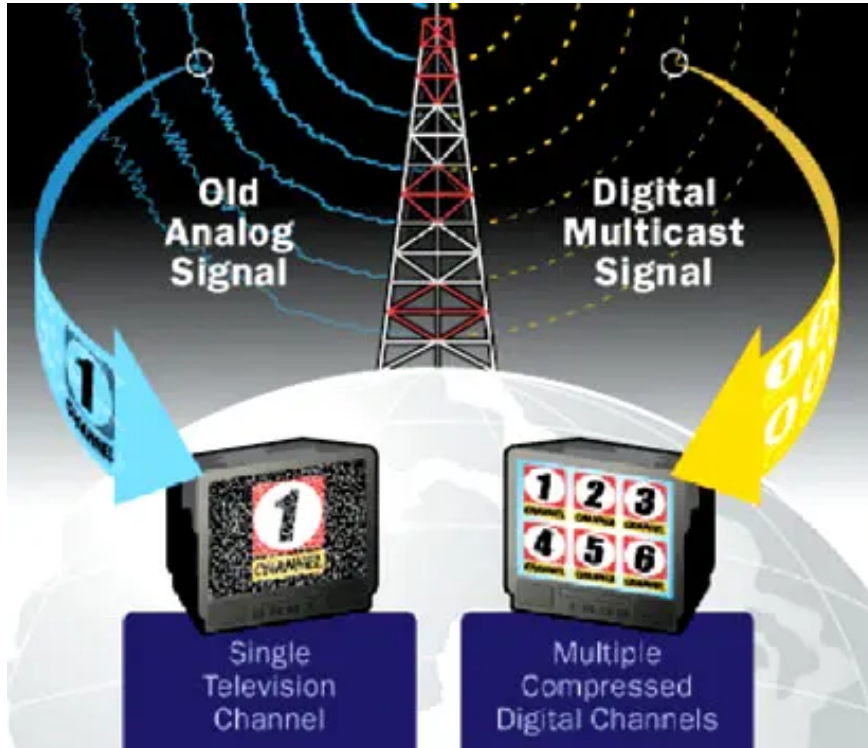
Figure 5. The difference between analog broadcasting and digital broadcasting.
