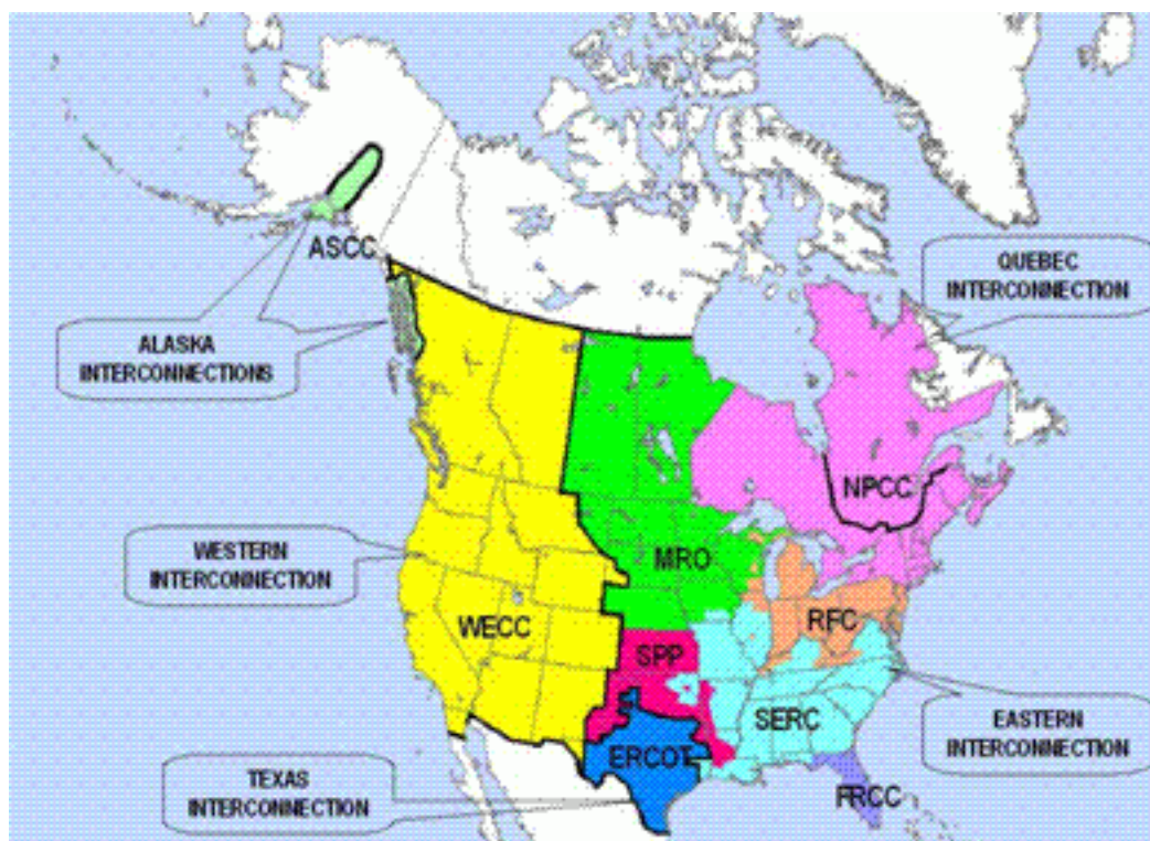
Figure 2: The various macro grids that power North America (Learn more about interconnections, n.d.).
